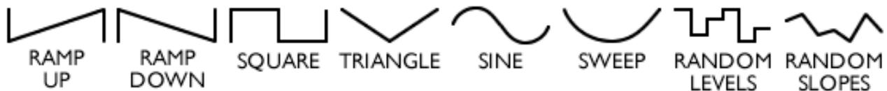
Some of the most exciting additions are the random waveforms. The Random Levels waveform is the classic “Sample & Hold” effect from analog synthesis and can produce early Sci-fi “computer thinking” noises amongst others.
